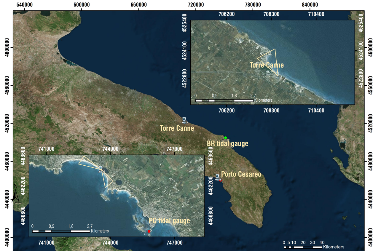
Figure 3.2 New Video Monitoring station installed at Apulia region: Camera locations and approximate Field of View (FoV). Nearest tidal buoy (dots) of Apulia monitoring network , BR: Brindisi; PC: Porto Cesareo . Grid coordinates: RDN2008/TM33.
