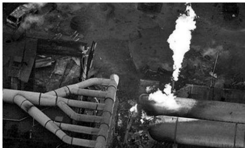
Figure 5.3 Image of a jet fire
