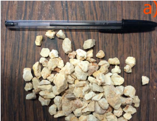
Figure 86 Sample of the material used for the experiments with different average grain size d_p . a) d_p = 9.2 mm b) d_p = 41.6 mm.
