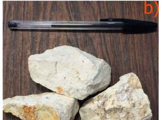
Figure 86 Sample of the material used for the experiments with different average grain size d_p . a) d_p = 9.2 mm b) d_p = 41.6 mm.
