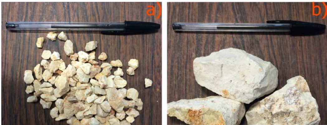
Figure 87 Sample of the material used for the experiments with different average grain size d_p . a) d_p = 9.2 mm b) d_p = 41.6 mm.
