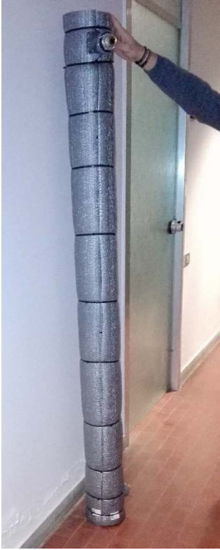
Figure 85 Thermal Insulated cylinder
