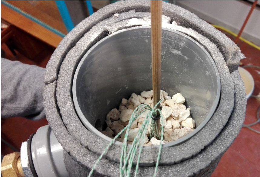
Figure 84 Thermocouple that have been equally placed along the axis of the pipe.
