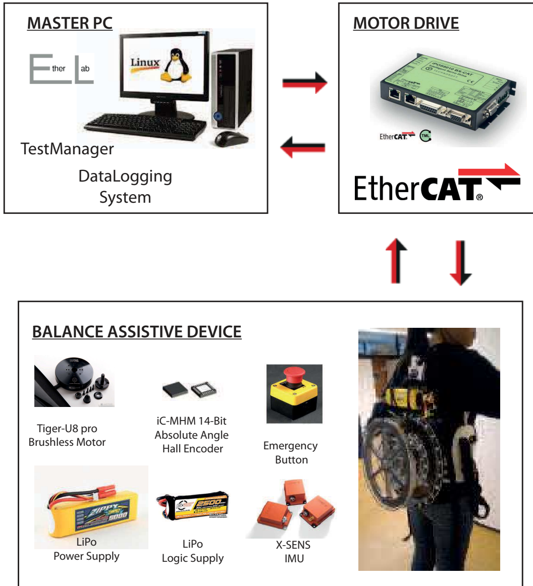
Figure 4.5: Scheme of the master/slave connection of the hardware components included into the flywheel inertial actuator. The arrows indicate the network connection among master/slave devices.
