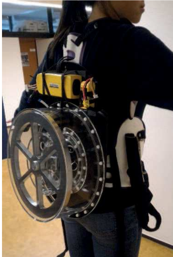
Figure 4.2: Flywheel inertial actuator for balance assistance. It weighs around 6 kg and its outer size is nearly 390 x 132 x 520 mm (L x W x H).
