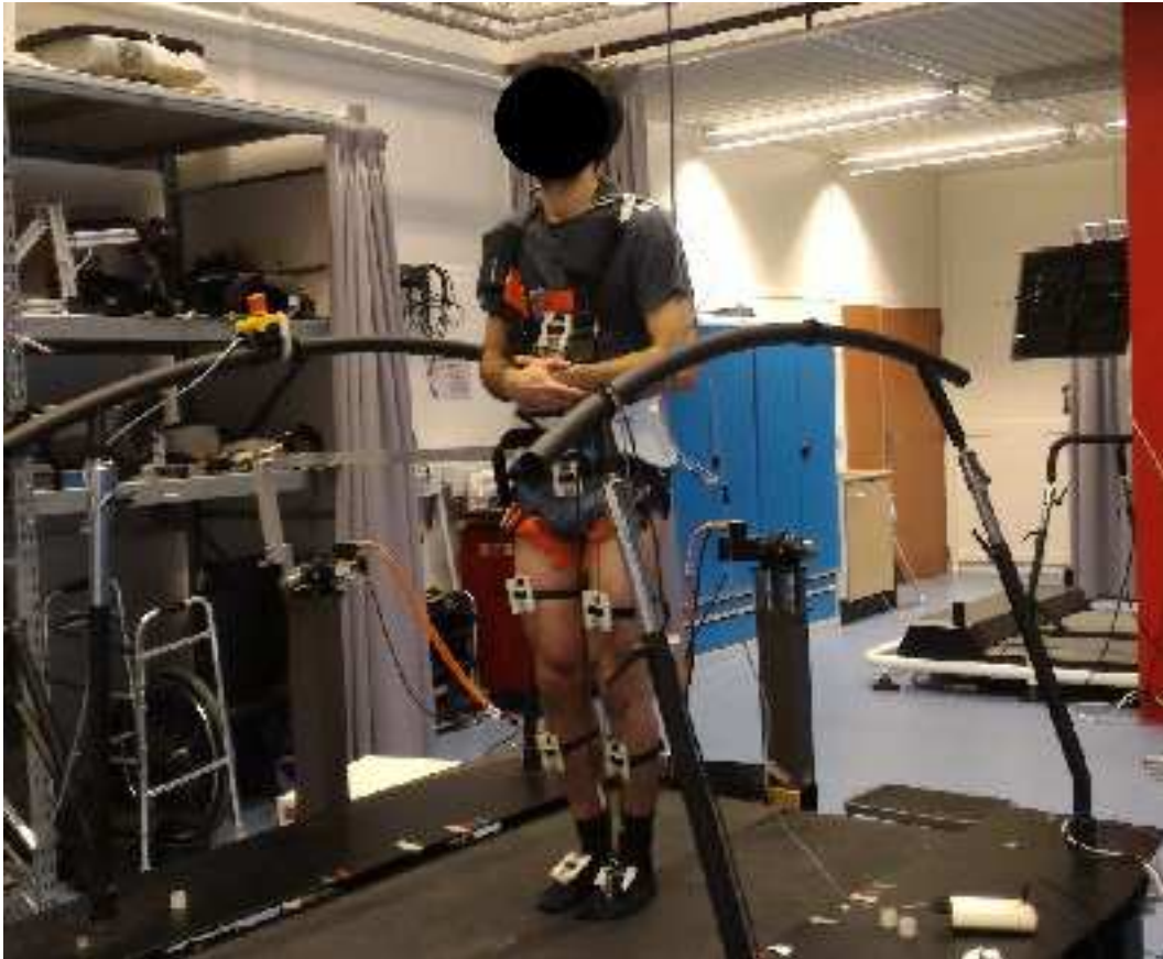
Figure 4.9: Experimental setup to assess the how the flywheel inertial actuator affects human balance. During experiments subjects were instructed to stand with bare feet on a treadmill including force plates, keeping their arms close to the chest to avoid any balancing effect. The subjects were attached to the pelvis perturbation system using a pelvis belt, and to a safety harness to prevent them from falling down if they were not able to keep balance by themselves.
