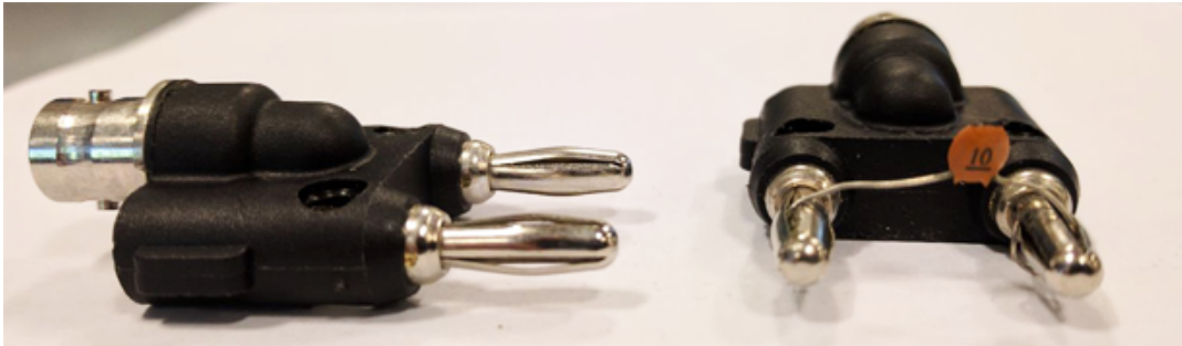
FIGURE 6.11: “F1” (left) and “F2” (right) capacitive fault devices
