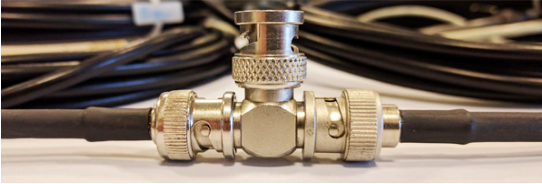
FIGURE 6.10: Junction between 5 m long RG58-CU coaxial cables
