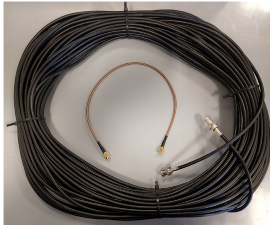
(a) Photo of a 50m long RG58-CU coaxial cable (DUT) and a 30cm long RG316 coaxial cable (connector)
