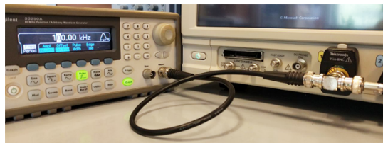
(b) TDR setup with an Arbitrary Waveform Generator (pulse signal with \sim 10 ns width) and an oscilloscope channel
