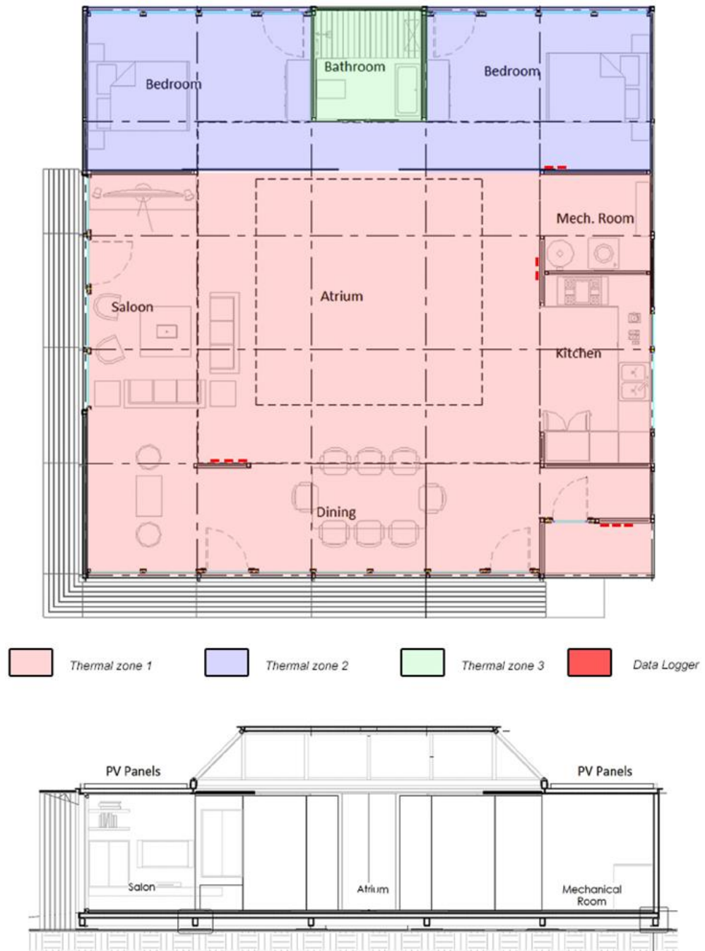
Figure 10: Solatrium plan-view (above) and section-view (below).
