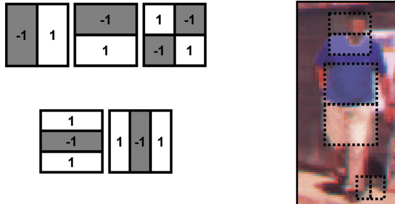
Figure 8: A representation of some filters from the extraction of Haar-like features from images. A contribution from [76].
