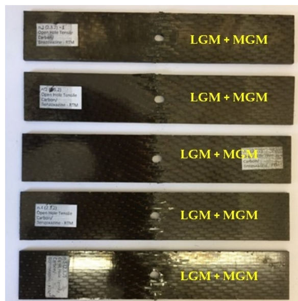
Figure 15. Open Hole Tensile Test: Carbon/Benzoxazine failure modes of specimens
