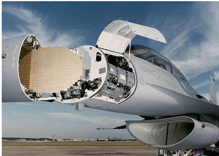
Figure 1.22 – Phased array radar inside the nose of an aircraft
