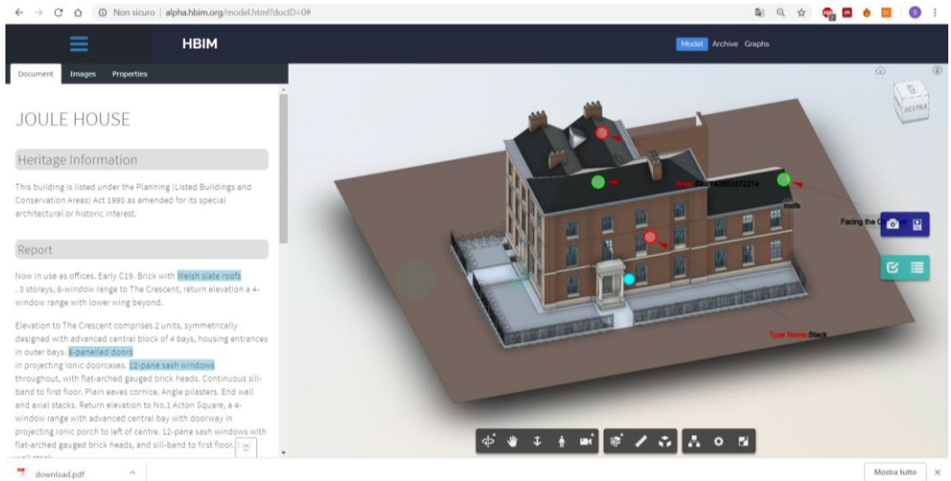
Figure 4.8-2 The reports viewer displays physical measurements, visual surveys, historic information, and analysis results.
