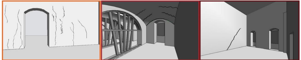
Figure 4.5-9 Selection of categories, property to be analysed, query and property value of the tree units. Down the cracking pattern of three rooms of the building, two on the ground floor (a)Unit 1 and (b)Unit 2, and one on the first floor (c)Unit 3.
