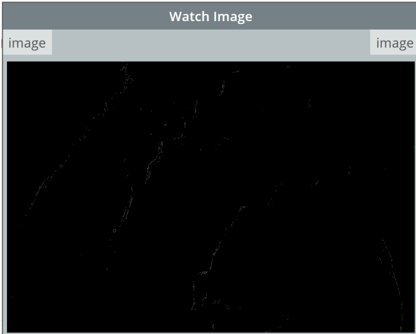
Figure 4.5-14 Test 2 run with Canny-Sobel filters: step 1 Canny. Source: author.
