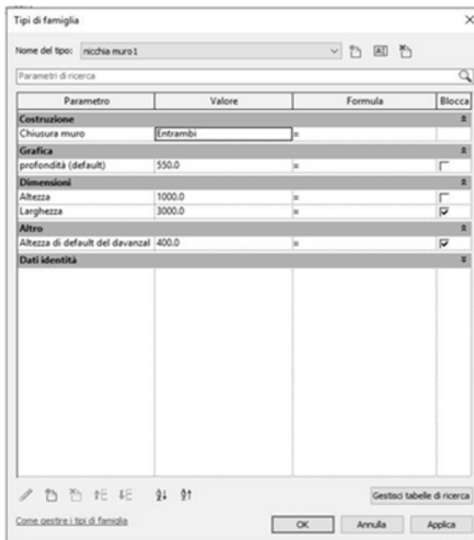
Figure 4.3-7 Masseria Macchia Trappeto. Parametric modelling of openings and niches. Source: (Modugno et al., 2016).
