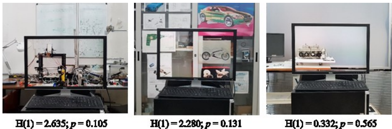
Figure 23 - Setup of the test with the monitor placed in front of the real backgrounds, with their digital image displayed on it. The results of the Kruskal-Wallis test showed no significant difference between the two conditions.
