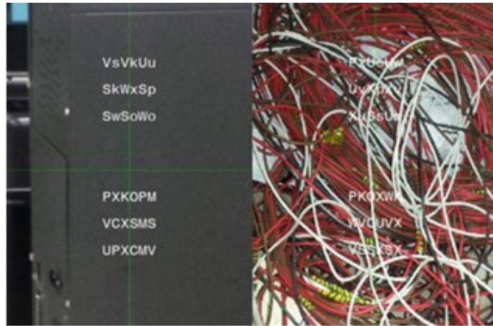
Figure 18 - The influence of the background in augmented reality: good legibility (left) and bad legibility (right).
