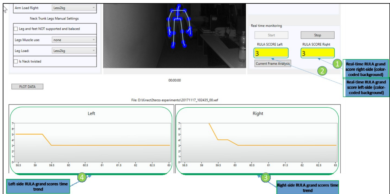
Figure 64 - The real-time feedback provided by the ERGOSENTINEL software, in the yellow boxes the real-time RULA grand score is visualized with a color-coded background.
