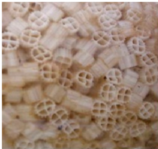
Fig. 2.5.2. Filling material kmt-k1 of Kaldnes.
