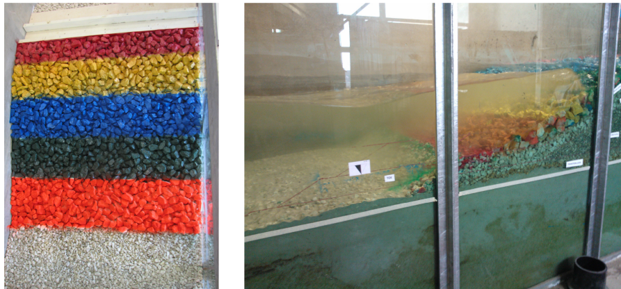
Figure 2.5: The experimental breakwater during the investigation.
