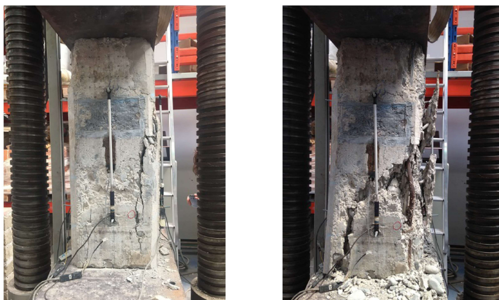
FIGURE 3.70: Damage states during the axial compression test: on left, second cycle state; on right, seventh cycle state
