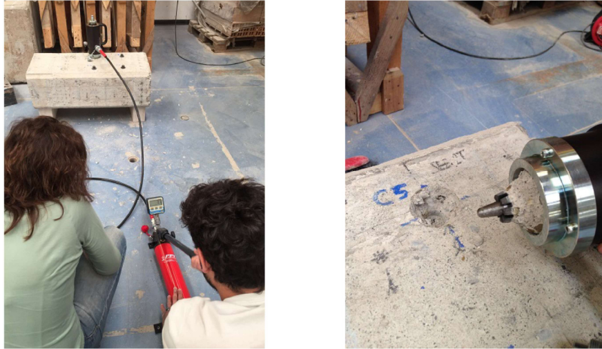
FIGURE 3.34: Pull-out test: on left side, testing execution; on right side, concrete sample extracted
