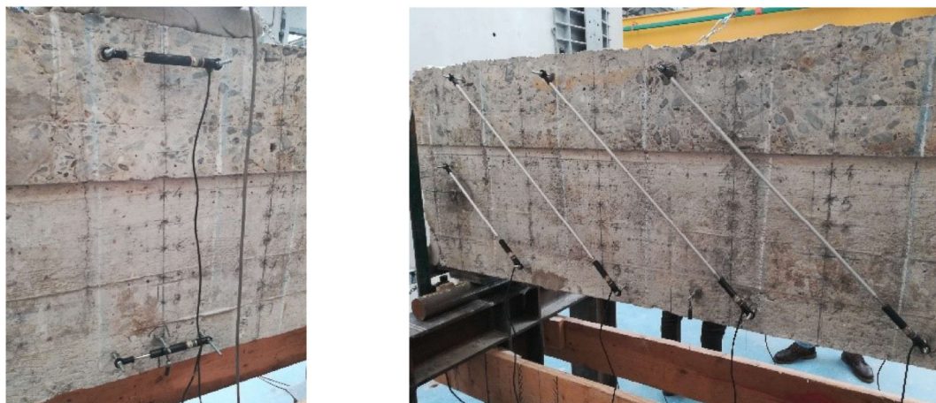
FIGURE 3.87: Potentiometers applied on portion of beam: on left side, horizontal type; on right side, diagonal type;
