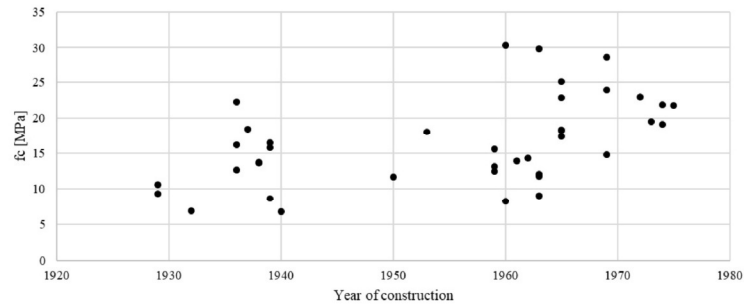
FIGURE 1.30: For each building, the mean values of compressive concrete strength according to year of construction
