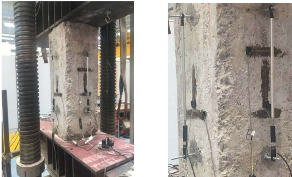
FIGURE 3.63: Technical instrumentation applied on portions of column
