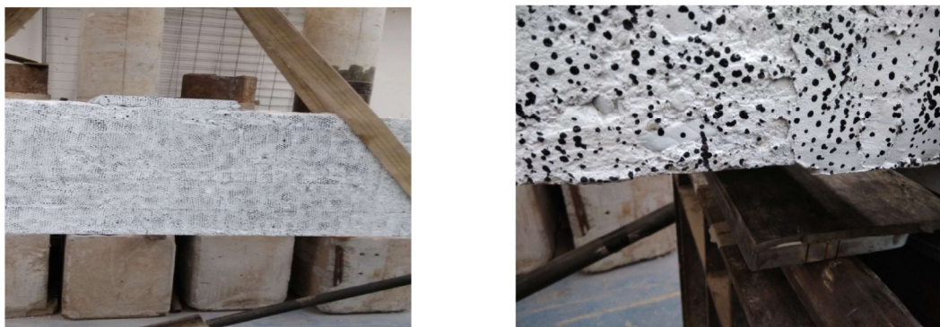
FIGURE 3.96: Speckle pattern used on portion of beam
