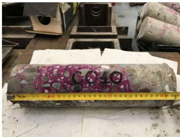
FIGURE 3.2: Phenolphthalein hydroalcoholic solution applied on concrete core
