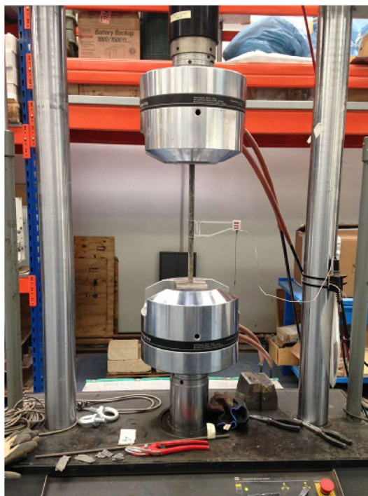
FIGURE 3.13: Tensile steel testing
