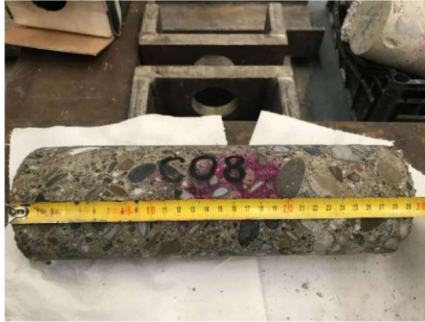
FIGURE 3.24: Phenolphthalein hydroalcoholic solution applied on concrete core C08 extracted from lower side of portion of beam
