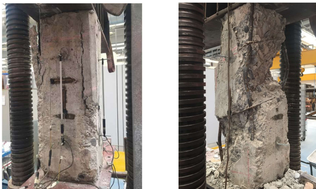
FIGURE 3.65: Damage states during the axial compression test: on left, third cycle state; on right, seventh cycle state
