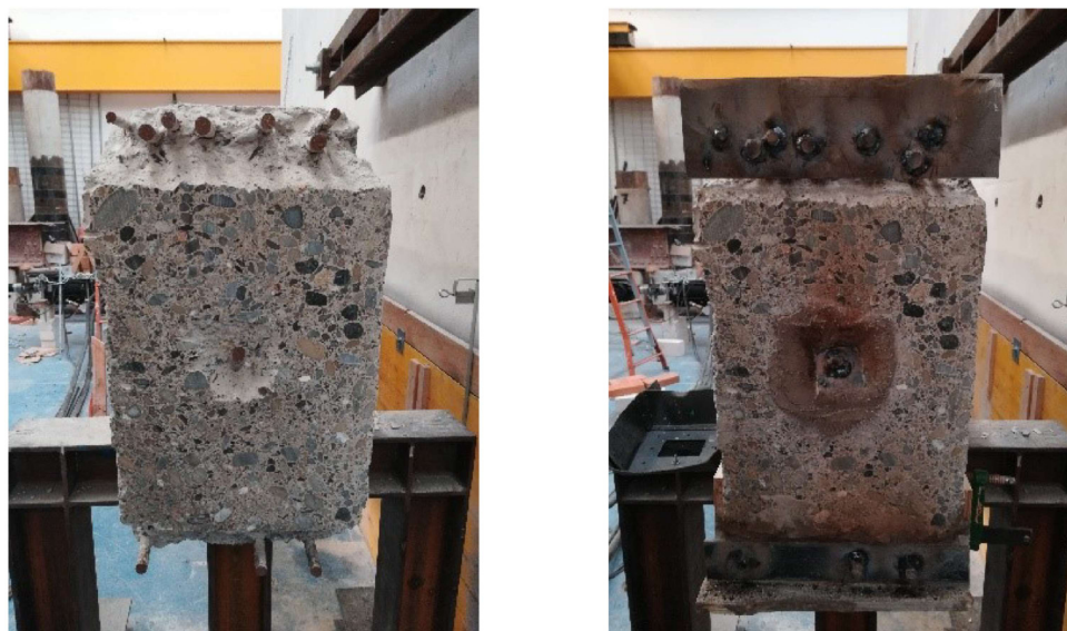
FIGURE 3.85: Longitudinal steel reinforcement fixing operations: on left side, concrete cover removing; in right side, steel plate welding
