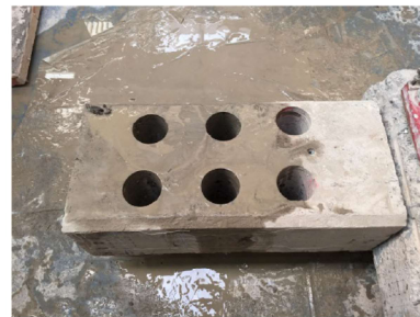
FIGURE 3.21: Concrete core extraction layout of top portion of column - floor I
