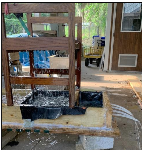
Figure 4-16 Picture of the ad-hoc self-development device for simulating the filtration process in PAS slab.
