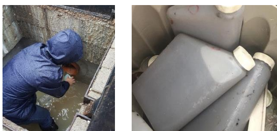
Figure 4-88 The author is sampling outflow water from the system (left) and some water bottle sampled (right).
