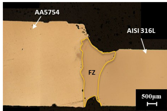
Fig. 70 Optical macrograph of cross section obtained by LOW technique [155].
