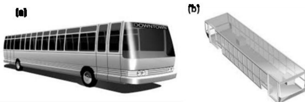
Fig. 26 (a) Ultralight Urban Bus and (b) Body structure [126].
