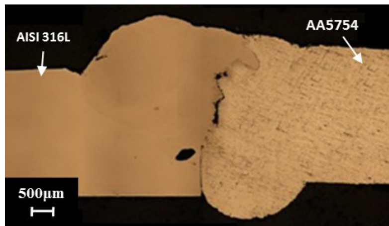
Fig. 79 Cross section by hybrid laser-MIG welding [155].
