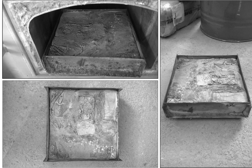
Figure 18 Obtained cast after melting and annealing phases.
