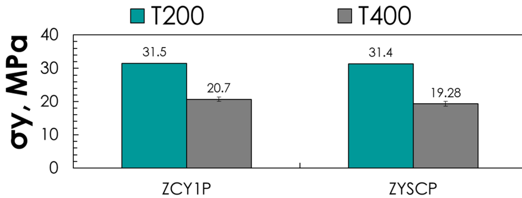
Figure 55 \sigma_y according to temperature for Mg-based alloy with three alloying elements.
