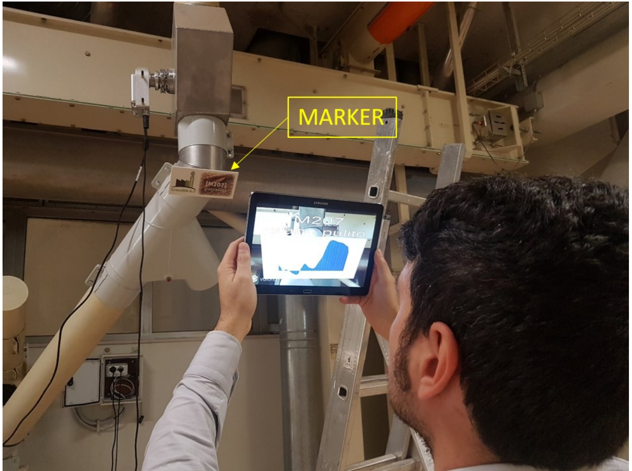
Fig. 3 An operator with a video see-through display, in particular a HHD (Tablet), framing a marker to augment the real scene.
