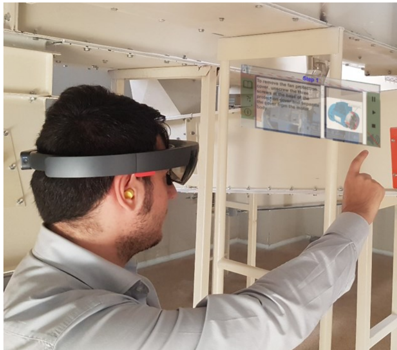
Fig. 42 Example of user interacting through (a) air-tap with the AR interface displayed on the HoloLens (AR interface added to the image in post-processing phase).
