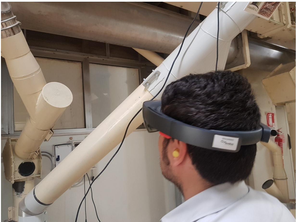
Fig. 2 An operator wears an HMD optical see-through display.
