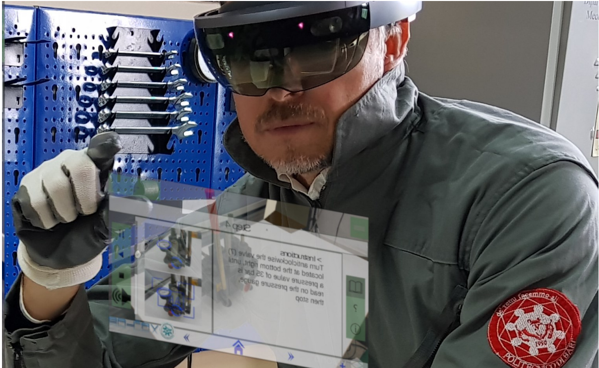
Fig. 6 Example of user interacting through air-tap with the AR interface displayed on the HoloLens (AR interface added to the image in post-processing phase).
