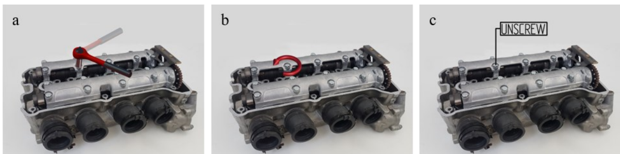
Fig. 1 Three different visual assets that convey the same instruction in an IAR interface: an animated product model of a socket wrench (a), a static auxiliary model of an arrow (b), a text instruction (c).
