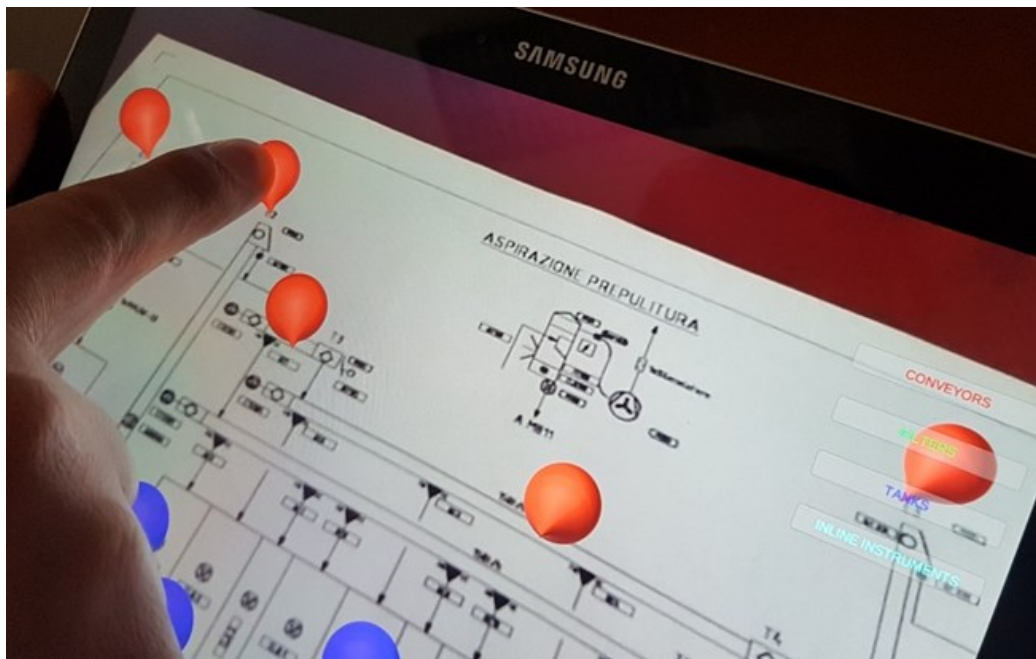
Fig. 36 User tapping on the hotspot to visualize the menu to access technical information.
