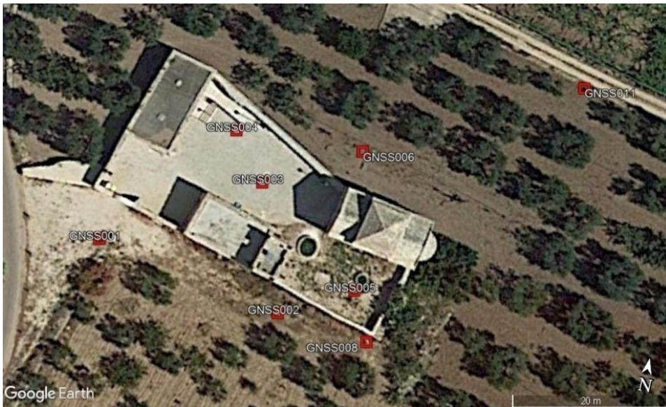
Figure 3.5. The test site and, in red, GCPs distributed in the area
