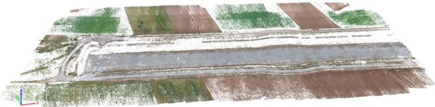
Figure 2.10. Sparse Points Cloud in Pix4D Mapper
