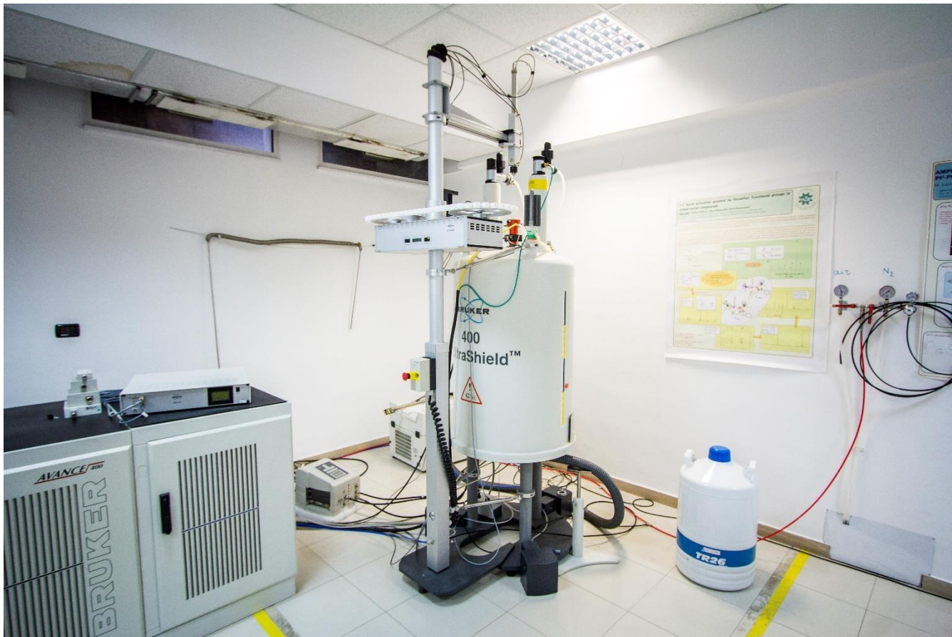
Figure 1. The Bruker Avance 400 spectrometer we used in most of our experiments
