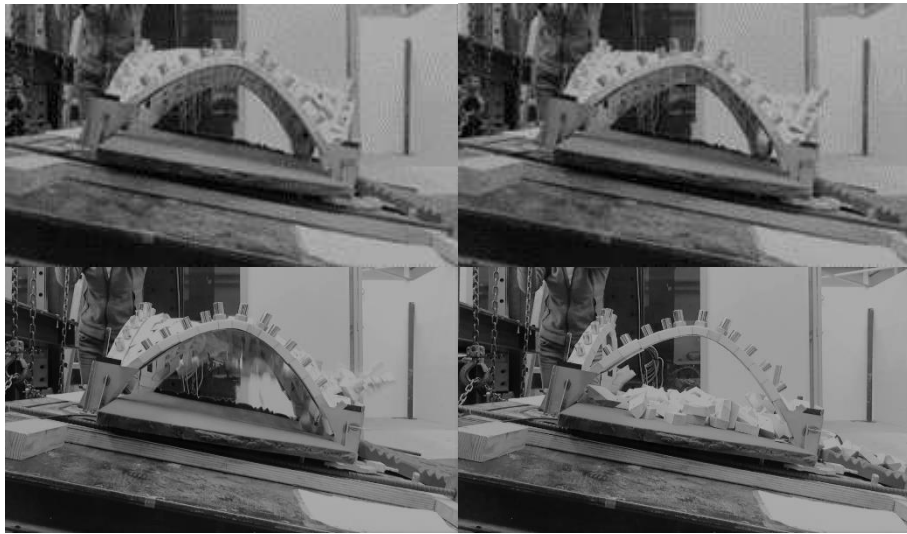
Figure 4-71. Damage results of the tilting tests with \Phi = 0^\circ : damage evolution in the lateral view ( p1-p3 ).
