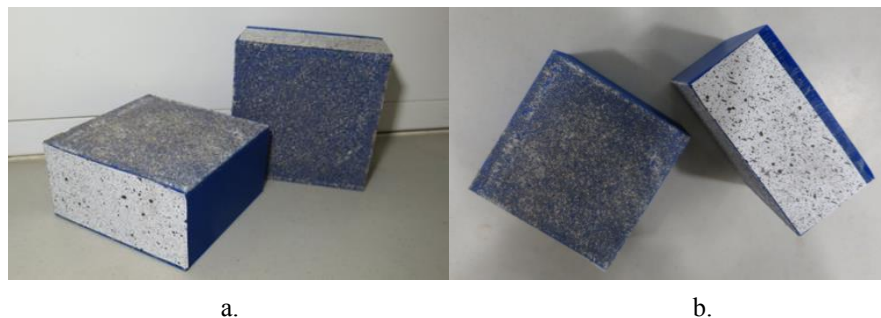
Figure 4-45. Example of specimens for shear box test: a. Later view; b. Top view.
