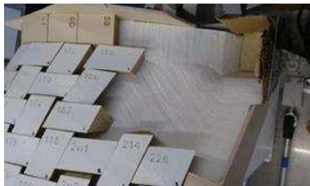
Figure 4-20. Interlocking between the blocks and contribution of the friction angle due to the sand coating.
