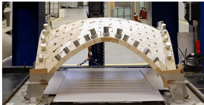
Figure 4-17. View of the vault after the disassembling of the scaffolding.
