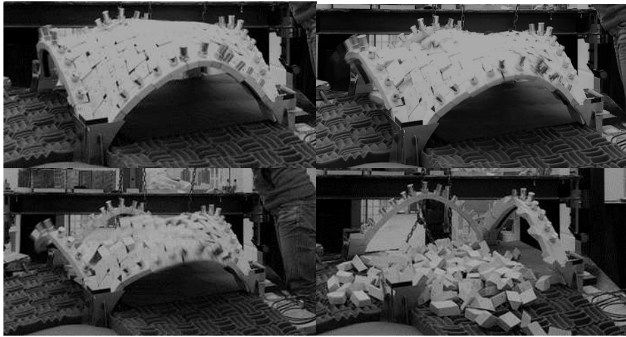
Figure 4-84. Damage results of the tilting tests with \Phi = 112.5^\circ : damage evolution in the frontal view ( p1-p3 ).
