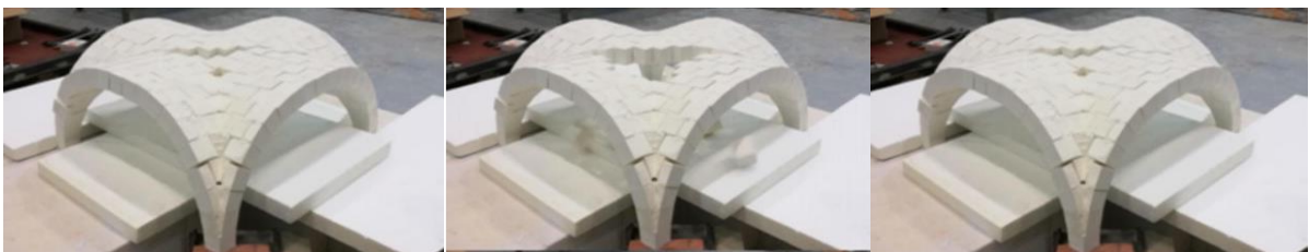
Figure 2-25. Progression of diagonal displacement test: collapse mechanism (D. Foti et al., 2018).
