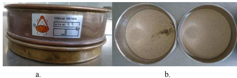
Figure 4-11. ATSM E 11-70 sieves: a. Meshes 40; b. Sand sieved with Sieve Mesh 80.
