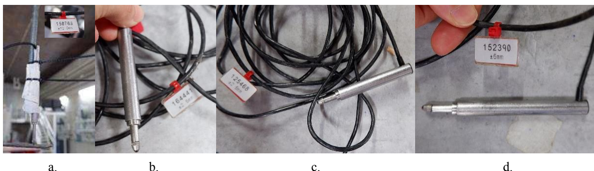
Figure 4-22. Linear Transducer Equipment: a. LTDV 156763; b. LVDT 164441; c. LVDT 125468; d. LVDT 152390.
