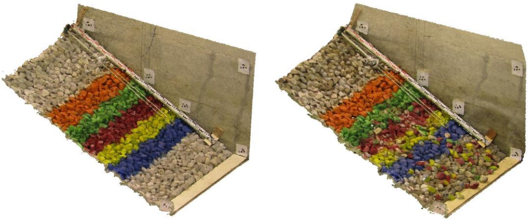
Figure 28 Example of point clouds pre and post wave test.
