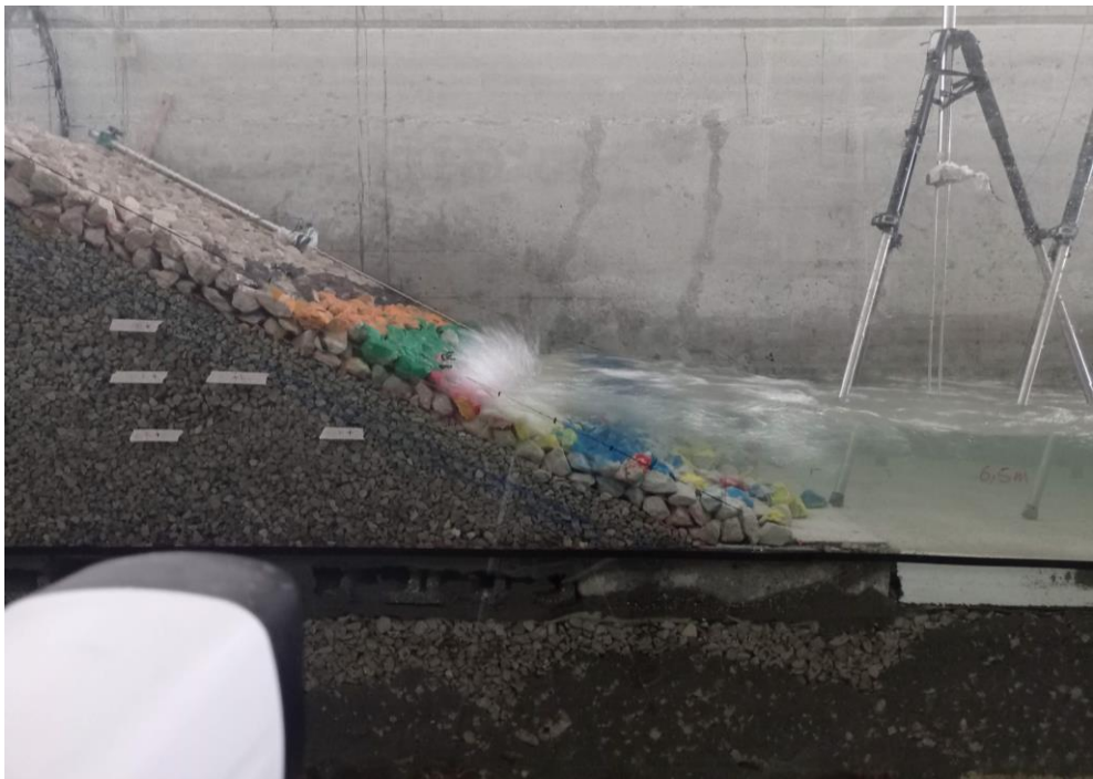
Figure 20 Wave impacting the rock armour slope.
