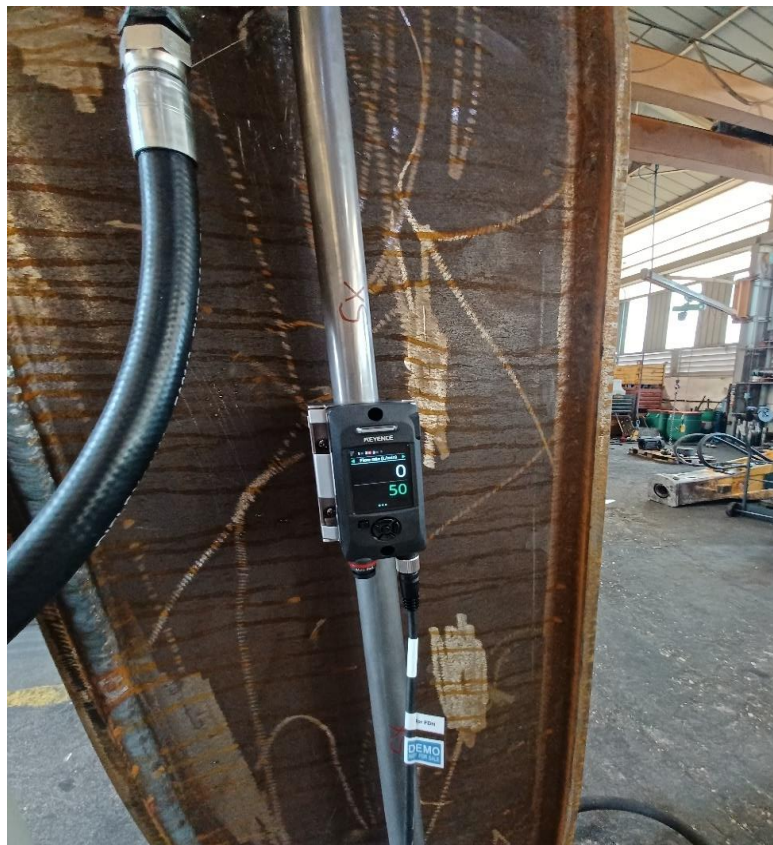
Fig 2- 9. Keyence FD-H series for monitoring the inlet of hydraulic hammers in the Indeco test bench house.
