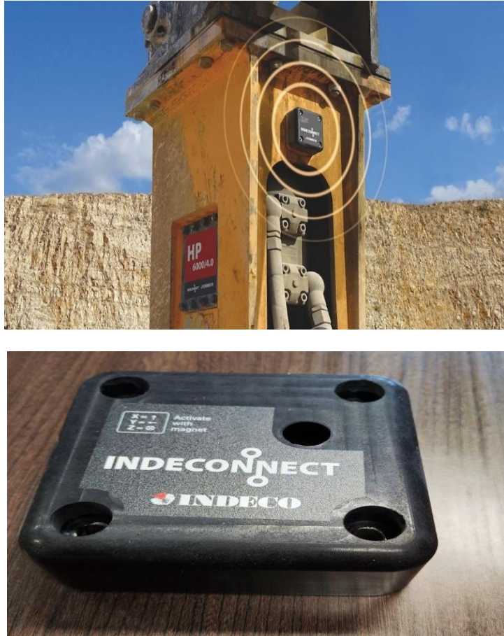
Fig 2- 13. the positioning of the data logger on the hydraulic equipment and the protective cover for the data logger.
