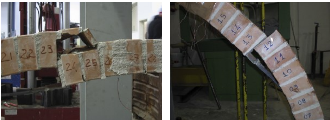
Figure 17: Collapse mechanisms (crushing, sliding or debonding) for a reinforced arch with FRP [46]
