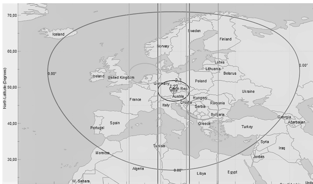
FIGURE 1.8: European field of view and satellite beam coverage.
