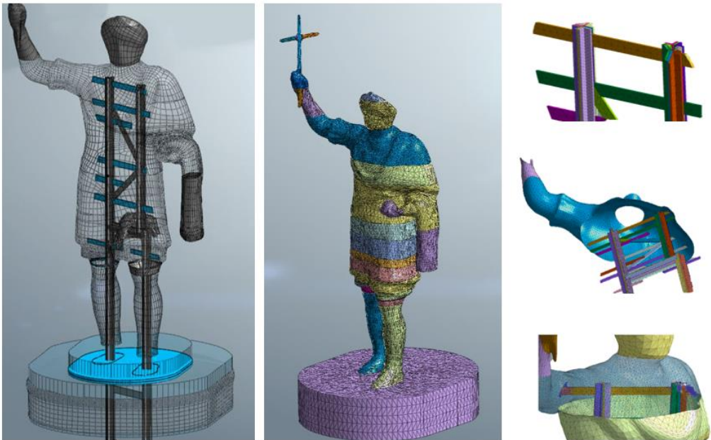
Fig. 6.14 - Modelling the connections between the bronze structure, the body and the steel structure.
