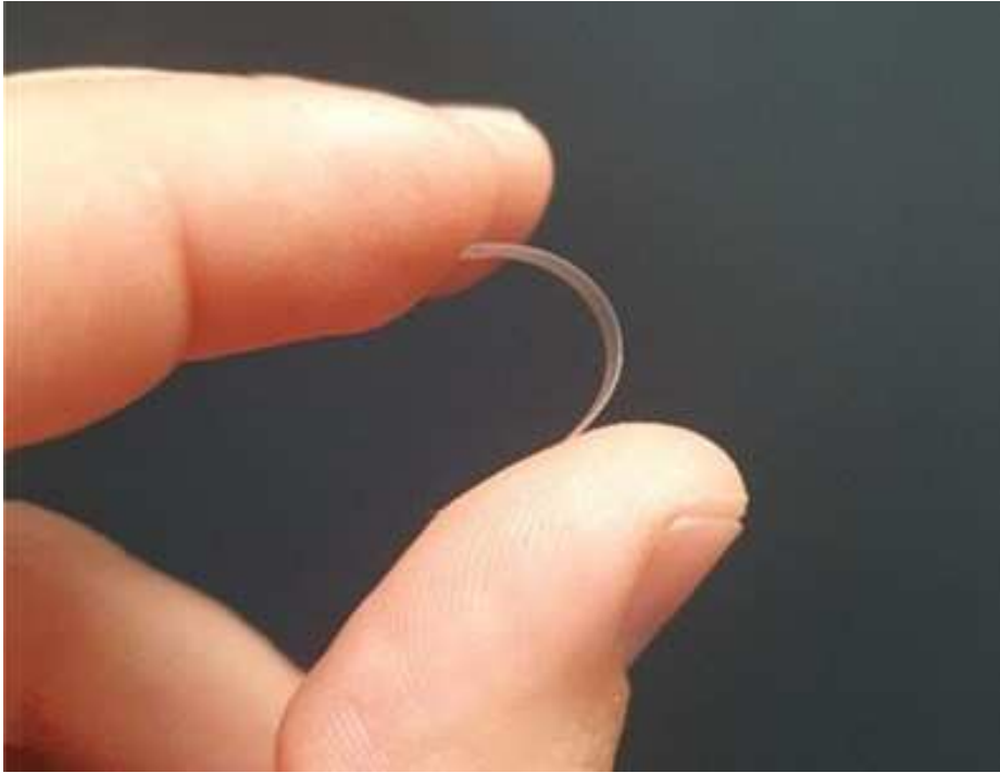
Figure 3.4.1 Flexible planar photonic chip in doped silica fabricated through Flame Hydrolysis Deposition [68].
