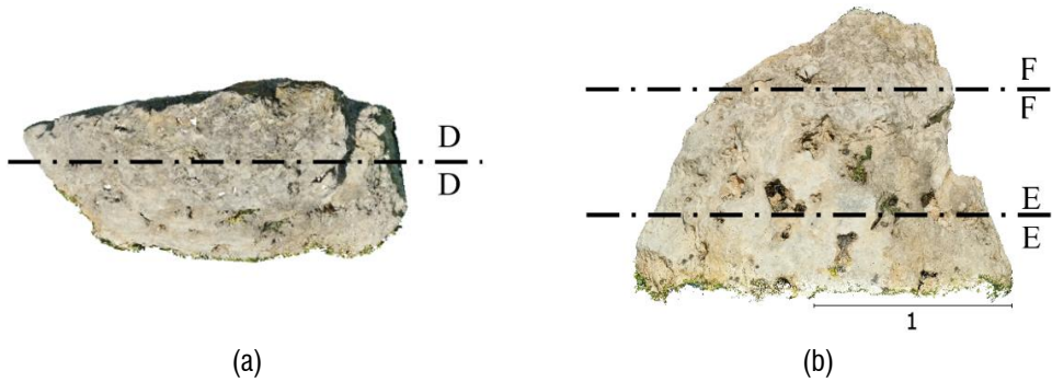
Fig. 45 – Point cloud of the ornamental garden boulder produced by the first approach: (a) plan section D-D, (b) plan sections E-E and F-F.
