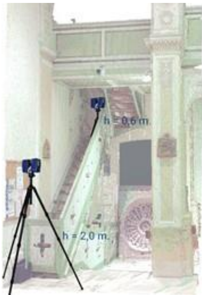
Fig. 17 Laser scanner stationing at different instrumental heights.
