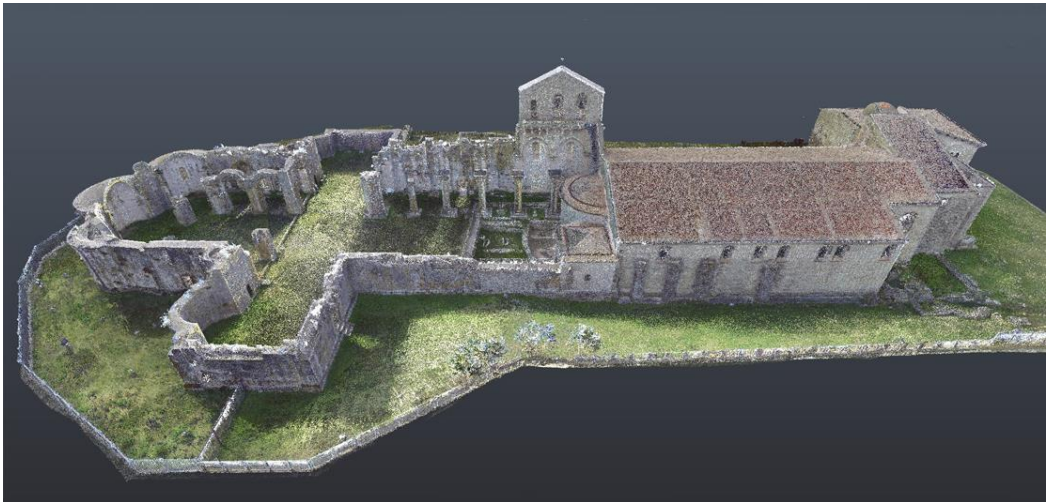
Fig. 47 Integrated point cloud of the entire complex.
