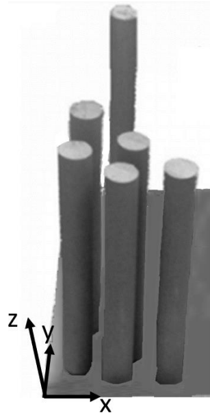
Figure 145 Distribution of the specimens on the building plate
