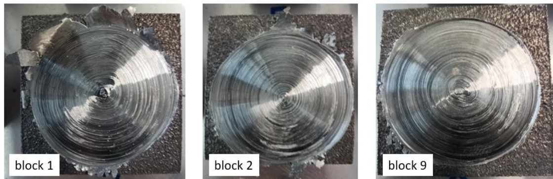
Figure 69 Deformation and flash in specimens processed with the combination of short dwell time and low rotational speed
