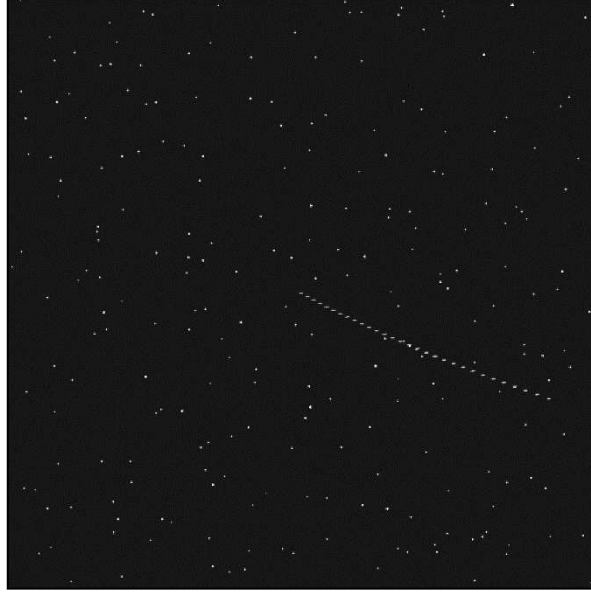
Fig. 4.2 Composite image obtained by superimposing successive captures of a transiting object, revealing its trajectory as a sequence of aligned dots
