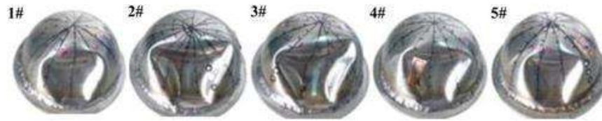
Figure 21: Collapsed hemispherical heads subjected to external hydrostatic pressure, exhibiting localized dimples as the characteristic failure pattern [64]
