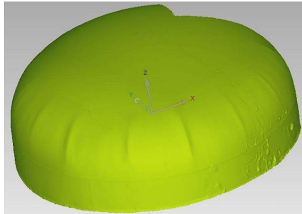
Figure 17: 3D Laser Scan Contour of Buckling Deformation [61]
