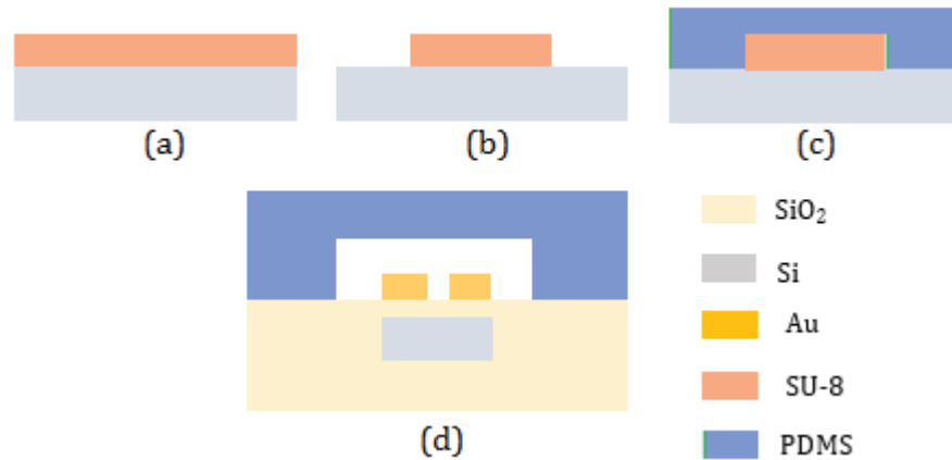
Fig. 6.6 (a-d) Fabrication process of the microfluidic channel used to integrate the hybrid cavity to realize the optofluidic chip.
