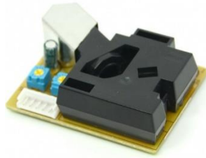
Figure 2.10: Grove - Dust Sensor
