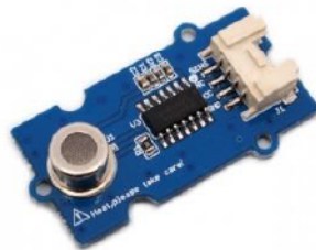
Figure 2.8: Grove - Air Quality Sensor
