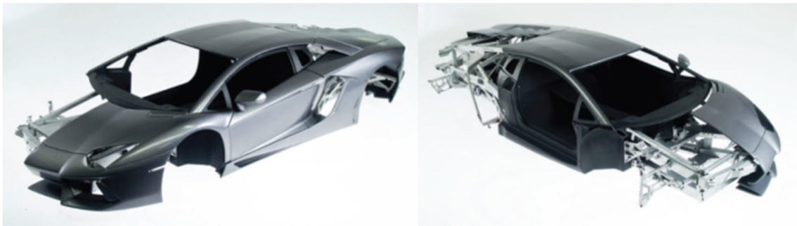
Figure 7.10 The 1/6 scale FDM prototype of Lamborghini Aventador
