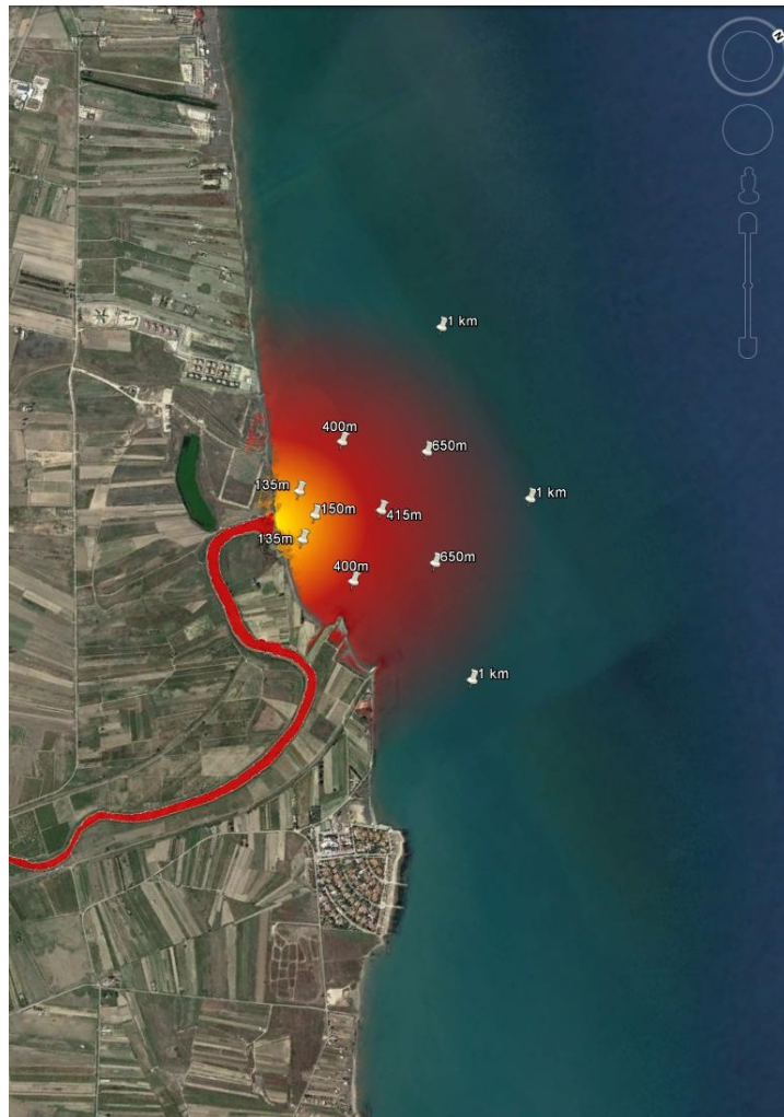
Fig. 10 Transitional water monitoring: Radial probe distribution (white) for impact zone detection. Example of chlorophyll- a (red) and inverse salinity (yellow) gradient maps that can be obtained.
