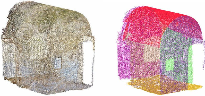
Fig. 69 Application of the RANSAC to the dense point cloud of barrel vaulted architectural unit of the Cappuccini ex-convent.
