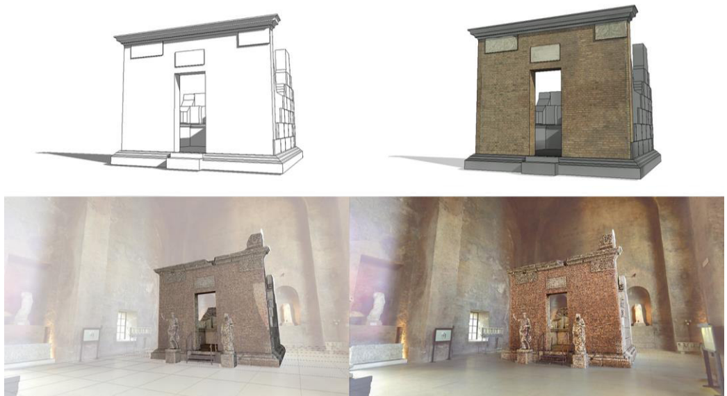
Fig. 38 On the top: (left) Parametric model at low LOD, (right) medium LOD; Bottom: (left) medium LOD model placed in the space, (right) High LOD (Verdoscia et al., 2021a).
