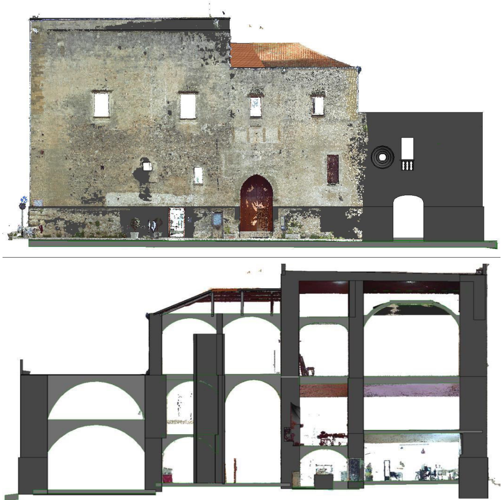
Fig. 91 The overlap of point cloud and 3D representation in BIM environment of Marchesale Palace of Laterza (Italy).
