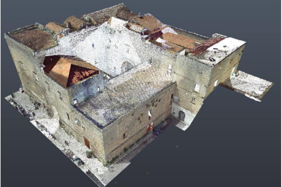
Fig. 81 The whole point cloud of the building resulting from data processing and filtering activity
