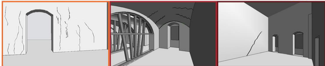
Fig. 99 On the top Selection of categories, property to be analysed, query and property value of the tree units. Bottom the cracking pattern of three rooms of the building, two on the ground floor (left) Unit 1 and (centre) Unit 2, and one on the first floor (right) Unit 3.
