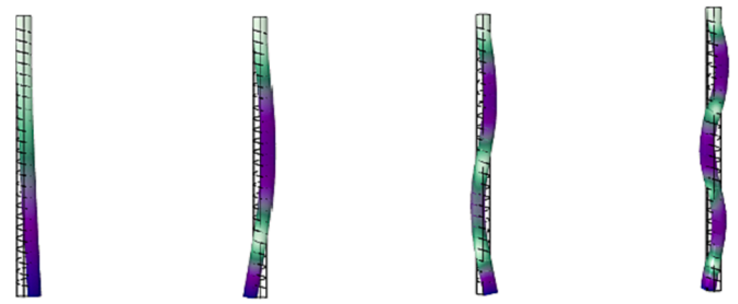
Fig. 11. First 4 flexural modes of vibration of a cylinder tube with discontinuous helical slit.
