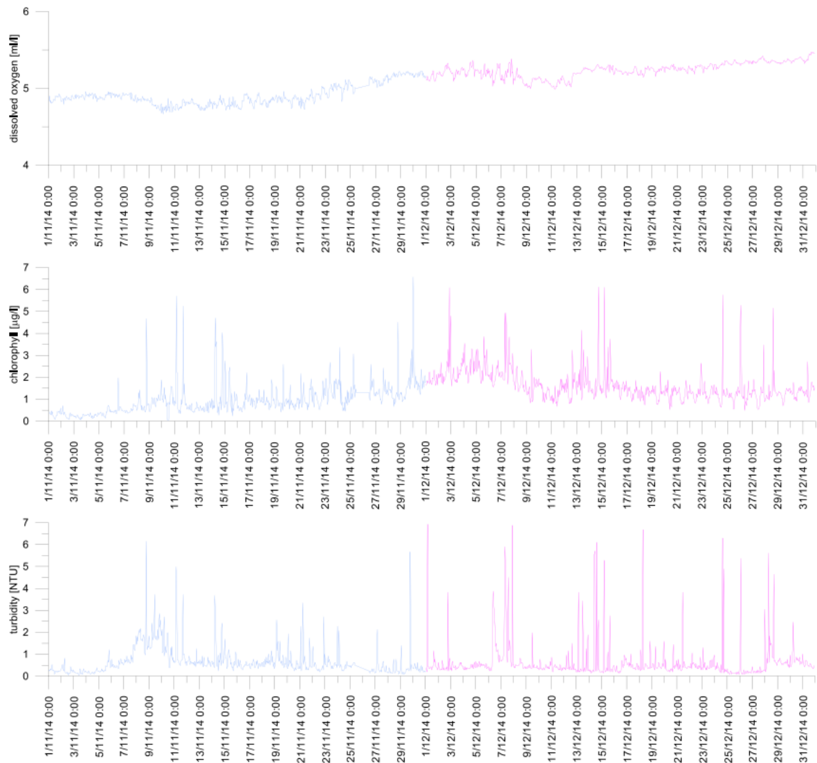
Fig. 8 Time series of dissolved oxygen, chlorophyll, and turbidity, during November and December 2014
