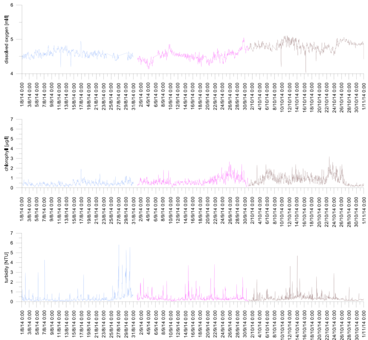
Fig. 7 Time series of dissolved oxygen, chlorophyll, and turbidity, during August, September, and October 2014
