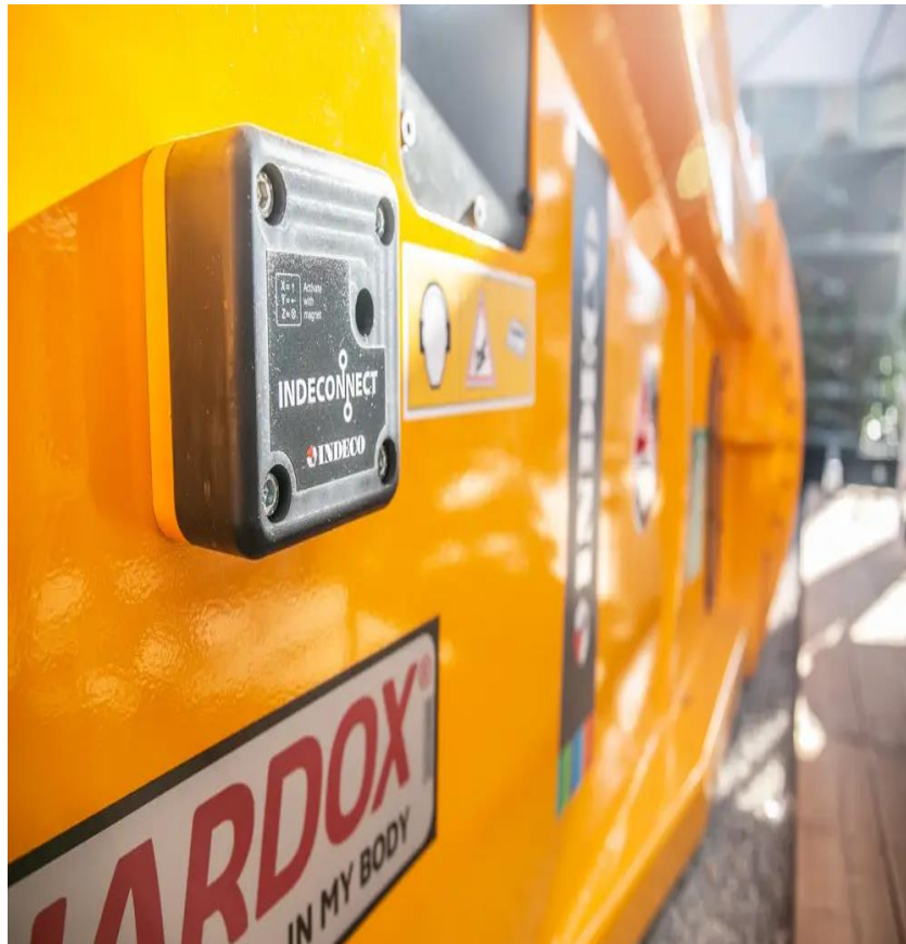
Fig 2- 2. Image and position of the INDECONNECT data logger on a hydraulic hammer INDECO HP 600 FS.
