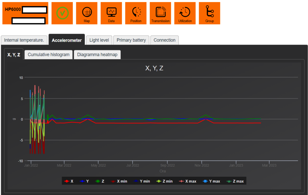
Fig2- 7. The accelerometer performance diagram for a hydraulic breaker model HP6000.
