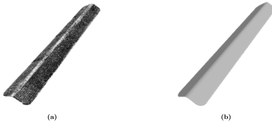
Figure 6.3: Comparison between the acquisition (a) and the CAD model (b) of a carbon angle profile
