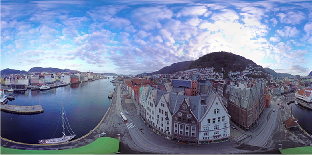
Figure 1.14: Omnidirectional scene in EAP format [2]. Please note as straight lines are curved.
