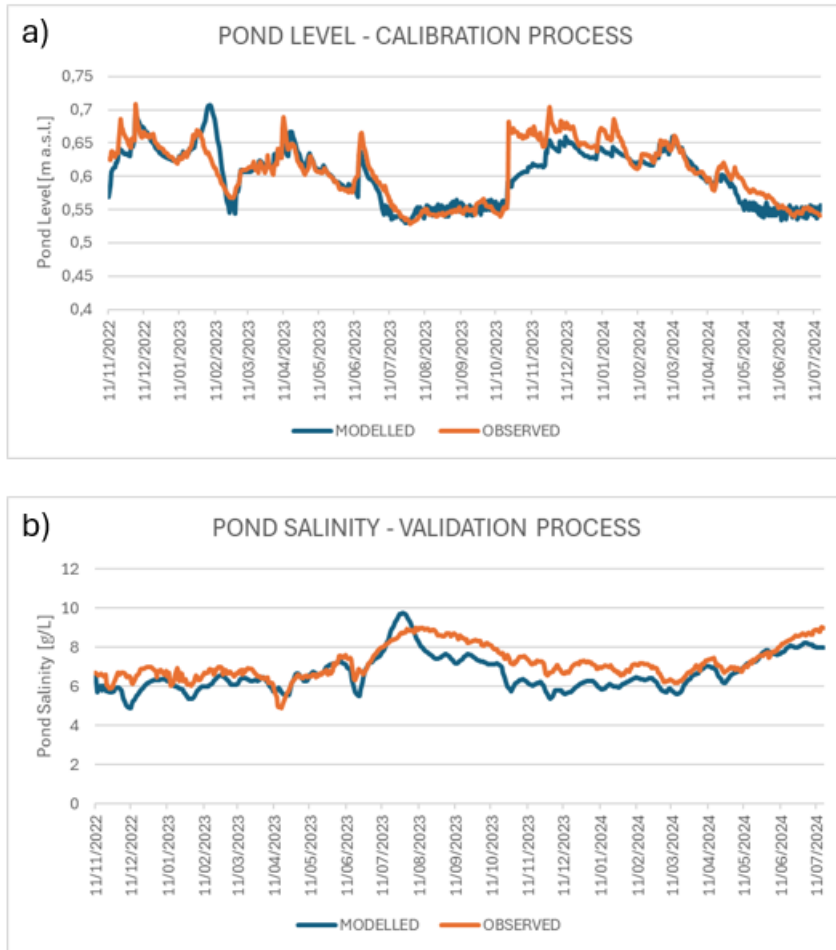
Fig. 33 – Panel (a) shows the WetMAT model calibration according to the “pond level” variable. Panel (b) shows the WetMAT validation process results according to the “pond salinity” variable
