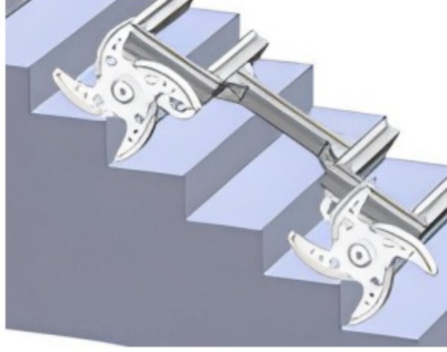
Figure 1.4: Krysl stair climbing robot in action [53].
