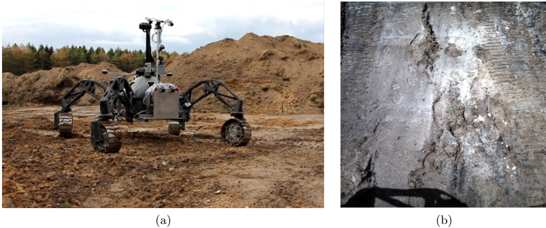
Figure 2.5.5.3: (a) Sherpa TT during the sand mine testing; (b) a close up of the tracks left by the wheels.
