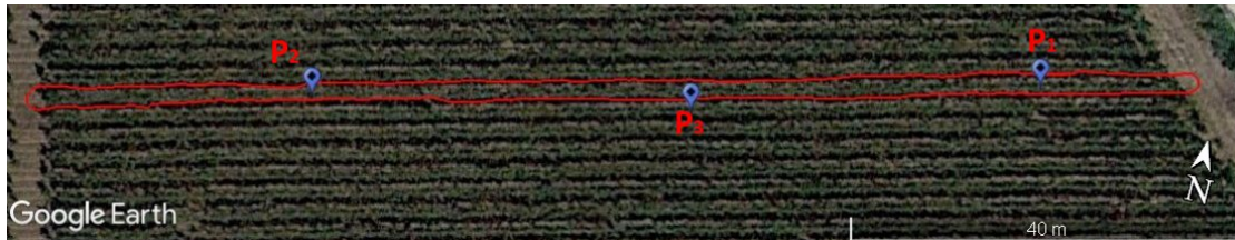
Figure 4.2.4.4: EIF-derived path overlaid on Google Earth view for Test 1. Three successive positions of the robot are pinpointed. For these positions, the corresponding visual data are shown in Figure 4.2.4.5.
