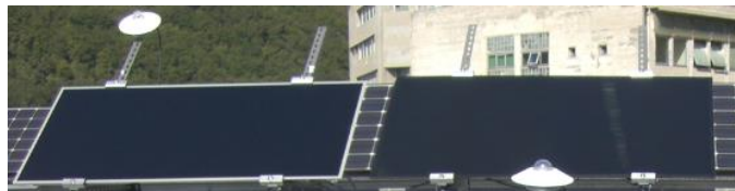
Fig. 2 The CdTe and CIGS PV modules used in the test
