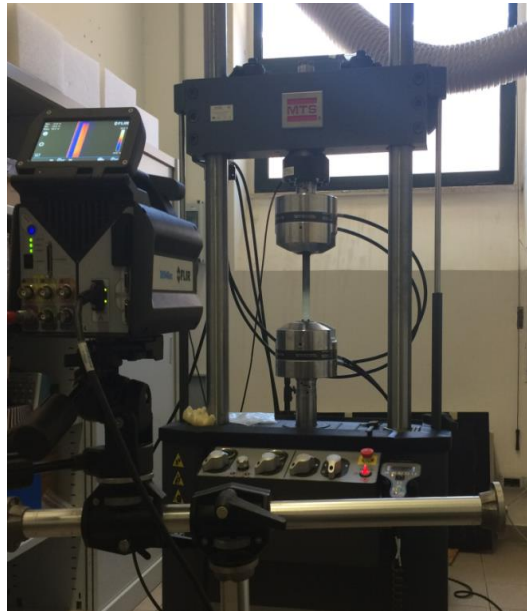
Figure1: Experimental set-up adopted for thermographic tests
