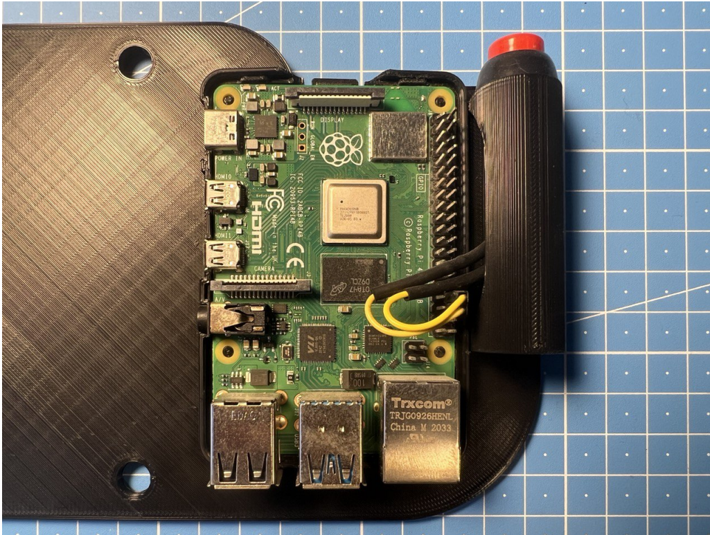
Figure 4.1: Experimental hardware setup with a Raspberry Pi 4 Model B mounted on a custom 3-D-printed bracket
