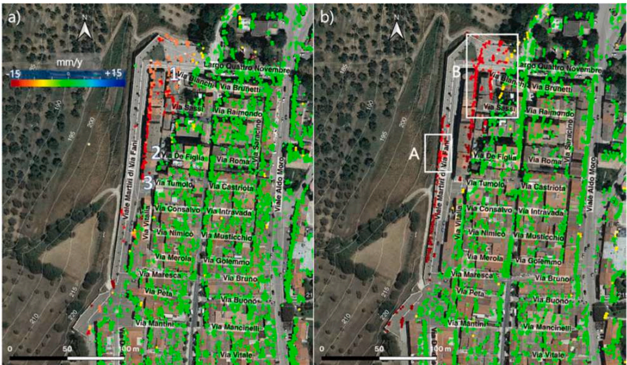
Fig. 4. a) Ascending and b) descending mean velocity maps resulting from the processing of the CSK datasets between January 2015 and December 2020, with a) the location of damages (1, 2 and 3) indicated in Fig. 7 and b) clusters A and B within white squares evidencing differential displacements.
