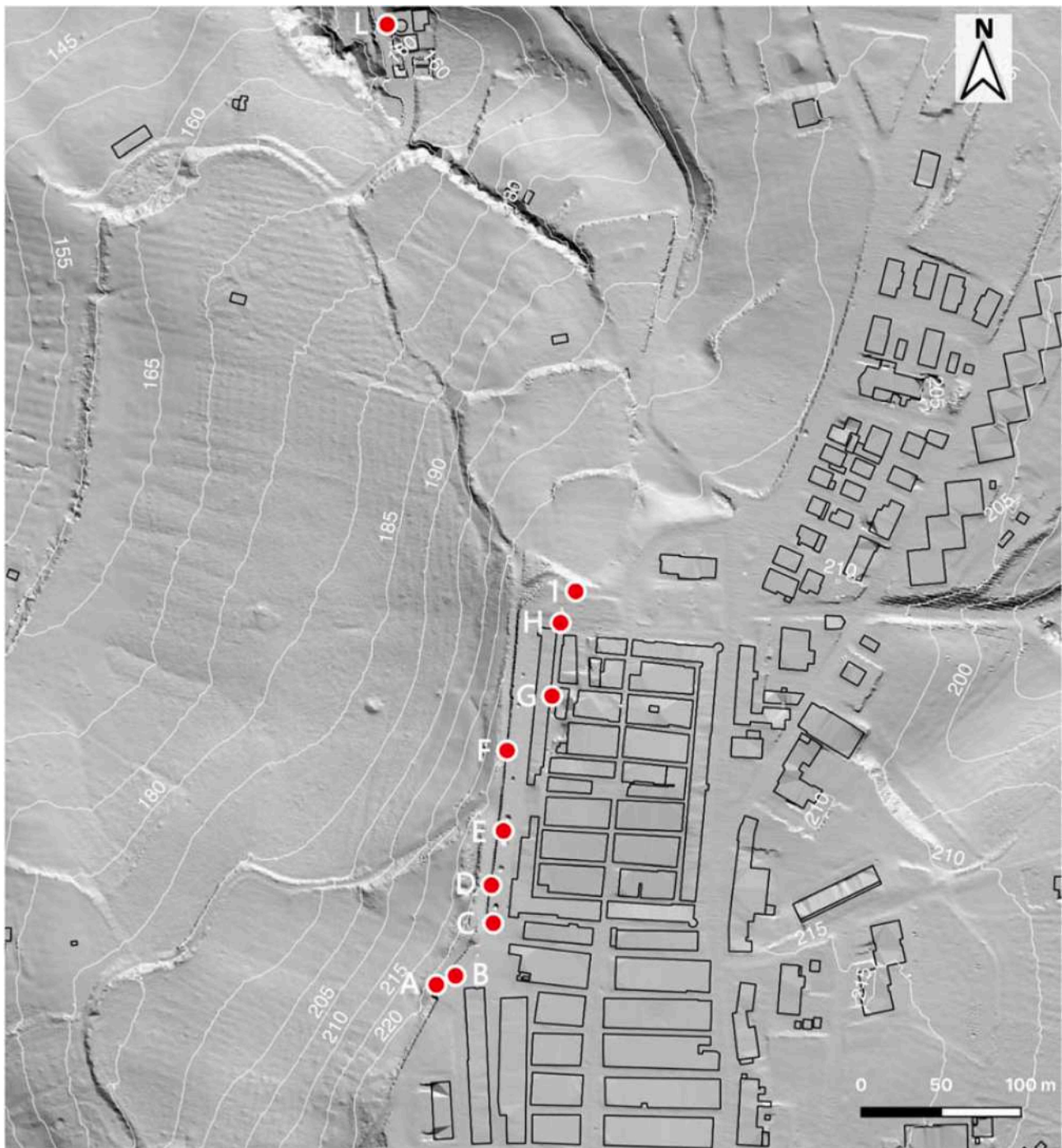
Fig. 8. High-coherence PS ( \geq 0.7 ) extracted from the CSK displacement map along the descending track. The red dots identify the targets investigated. (background: LiDAR Digital Elevation Model). (For interpretation of the references to colour in this figure legend, the reader is referred to the web version of this article.)
