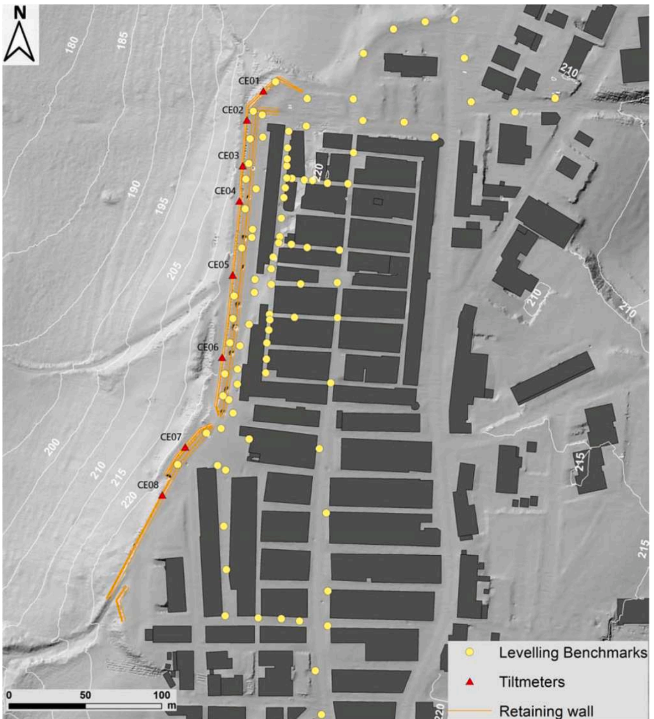
Fig. 17. Ground-based geomatic system monitoring the urban area (background: LiDAR Digital Elevation Model).
