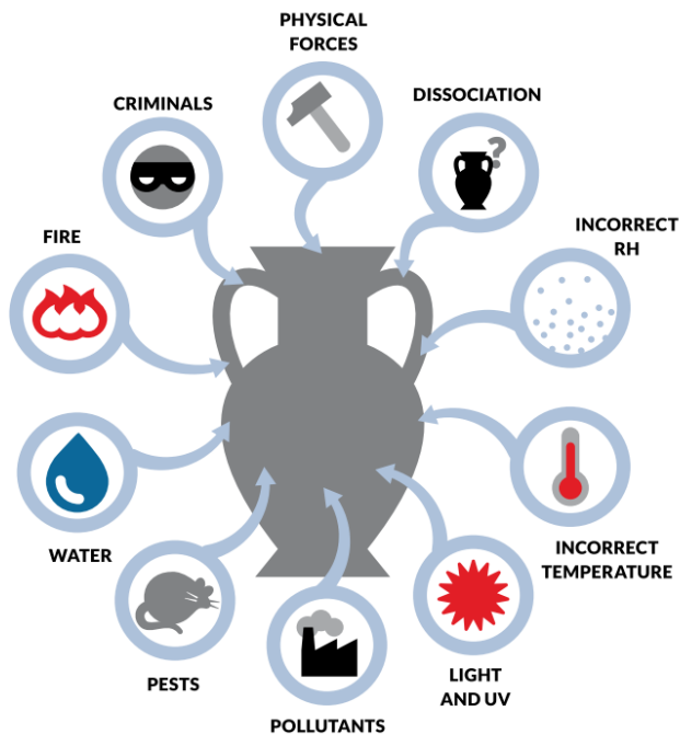
Fig. 1 Ten agents of deterioration and loss in heritage asset - Source (ICCROM, 2016)
